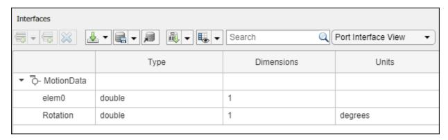
Connect components with an interface rule and the default name rule. The interface rule connects ports on components that share the same interface. By default, the name rule connects ports on components that share the same name.
