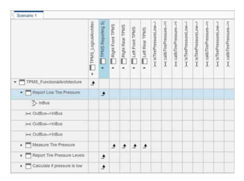
The arrows display allocated components in the model. You can observe allocations for each element in the model hierarchy.
