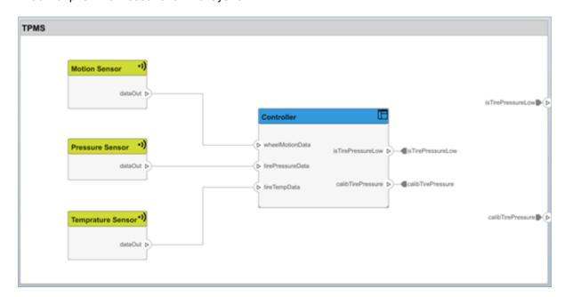
Open the FunctionalAllocation.mldatx file, which displays allocations from TPMS\_FunctionalArchitecture to TPMS\_LogicalArchitecture. The elements of TPMS\_FunctionalArchitecture are displayed in the first column. The elements of TPMS\_LogicalArchitecture are displayed in the first row. The arrows indicate the allocations between model elements.
