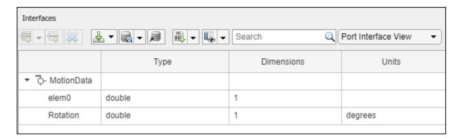
Connect components with an interface rule and the default name rule. The interface rule connects ports on components that share the same interface. By default, the name rule connects ports on components that share the same name.
